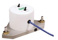
You can use Jewell Tiltmeters and Miniature Tilt Sensors to level platforms and equipment within a few microradians of true level. Here's how:
