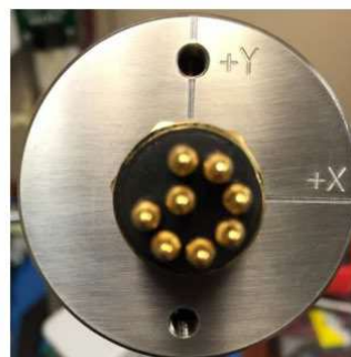
Figure 2: Male Bulkhead Connector showing +X & +Y axis Orientation (left) and Pin Number Orientation (right)
