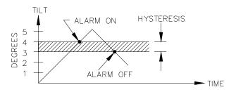
In standard IRIS models the control pins in connector H3 are all set high for approximately 150 milliseconds on power up, after which they reset to their "normally low" value of OV until a tilt threshold is detected.
