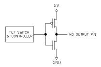
The standard IRIS firmware also allows the user to set the hysteresis of the control thresholds. The hysteresis is used as follows: After an H3 output pin is set high, it is not set low again until the tilt reading has reached a level that is below the threshold by an amount equal to the hysteresis (see diagram).
