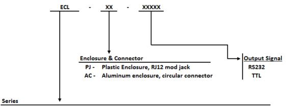
ECL - Electronic Compass with 3-axis magnetometer, 2-axis tilt sensor & low power 50  $\mu$ A standby
