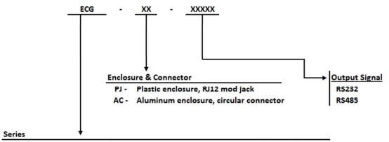
ECG - Electronic Compass with 3-axis magnetometer, 3-axis gyroscope & 2-axis tilt sensor
