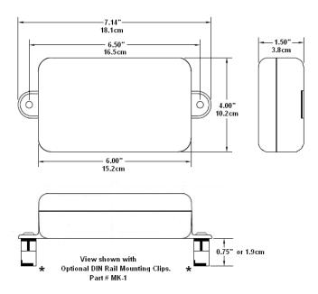
The D8000 series modules can be easily adapted to a DIN rail using the DGH MK-1 mounting kit shown in view above.
