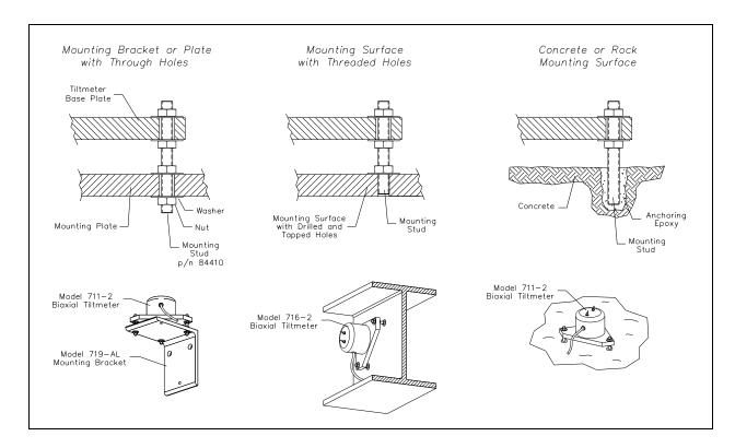
Figure B1. Installing Model D711 Digital Floor Mount Tiltmeter
