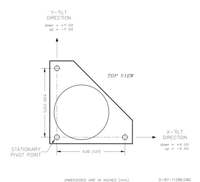
**Figure 3: Floor Mount Tiltmeter Sign Convention**
