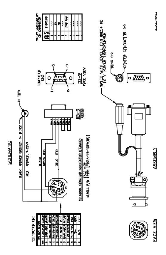
Figure 5: RS232 Test Cable (Part No. 89063) for Use with Model D711 Tiltmeter
