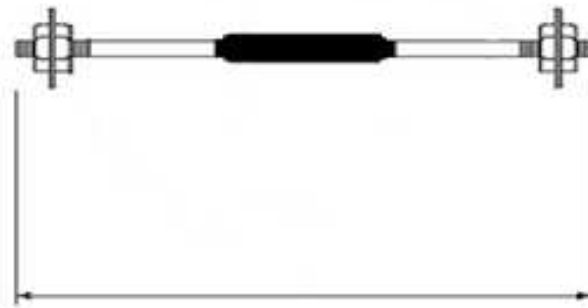
5/16" Diameter by 8" Long Sensor
