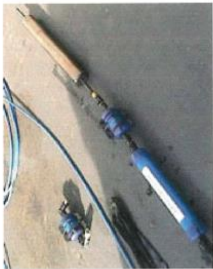
6. Lower-most Little Dipper/universal pivot/tensioning weight ready for installation
