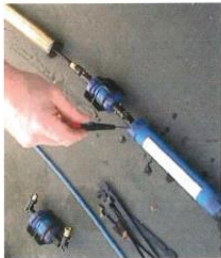
5. Tightening cap screw - tensioning weight already attached to bottom of universal pivot
