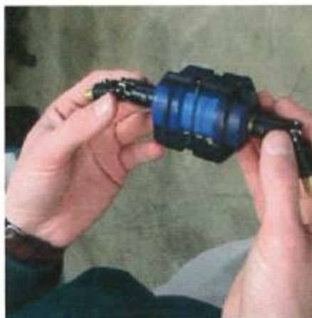
2. Universal pivot with cushion O-rings, guide fins and circumferential O-ring
