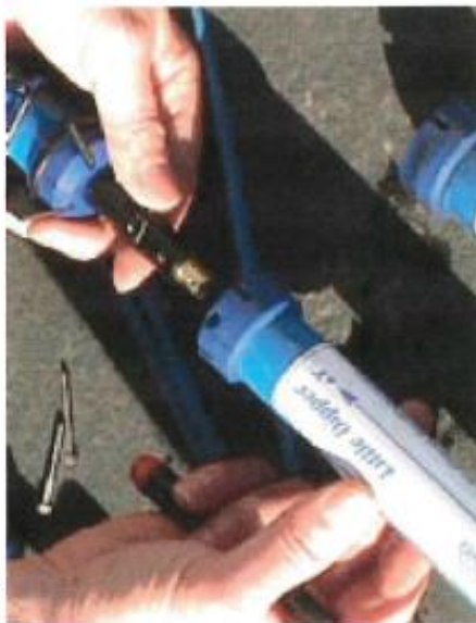
3. Aligning cross-hole in universal pivot with cross-hole on bottom end cap of Little Dipper
