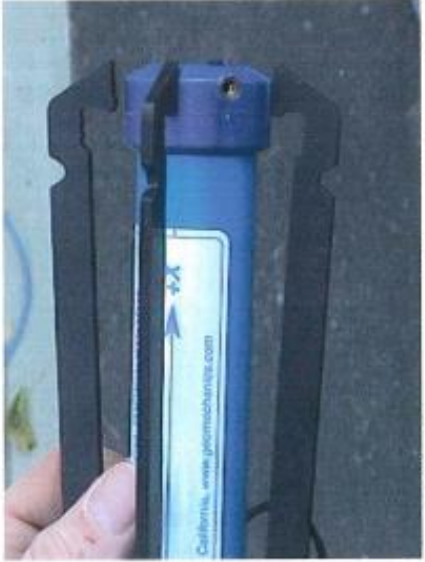
3. Guide fins removed for cushioning O-ring replacement
