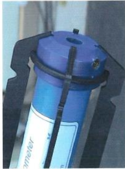
4. Cushion O-ring used to make guide fins fit snugly in casing
