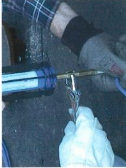
12. Screwing connecting rod into bottom of Little Dipper
