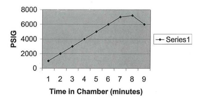
Pressure ramping was started at 2.15 pm. Chamber pressure showed linear response to nominally 7200 psi. Deepsea technicians noted a 1200 PSIG drop nominally 7 minutes into the test. Failure pressure was noted at nominally 7200 psi.
