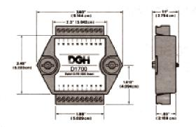
**NOTE:** Spacing for mounting screws = 2.700" (6.858 cm). Screw threads are 6 x 32.
